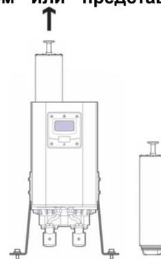
Fig.23-B: Dryer cartridge
